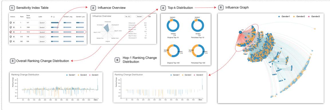
Figure 13. Facebook sensitivity analysis on PageRank. (1) The sensitivity index list shows that user 136 has the 4th largest influence on the Sensitivity Index while its ranking score is 312 out of 734 nodes, which is considerably low for such a large influence. (2) The influence overview shows that the removal of user 136 influences 644 of the 734 nodes, with 482 of them being positively influenced (ranking increased) while 162 are negatively influenced (ranking decreased). (3) The ranking change distribution view shows that negatively influenced nodes see a larger ranking decrease in comparison to positively influence nodes. (4) The top-k distribution view shows that as k increases from 10 to 100, the proportion of gender 2 increases, which means nodes of gender 1 are ranked relatively higher than nodes of gender 2. (5) The influence graph view further explains that most of those nodes who have large ranking changes are the neighbors of the removed user 136 , and (6) the corresponding distribution view shows that those neighbors’ rankings are evenly distributed.
