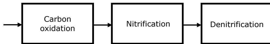
Figure 32 Separate Stage, Carbon Oxidation, Nitrification, Denitrification (Sedlak, 2001)
