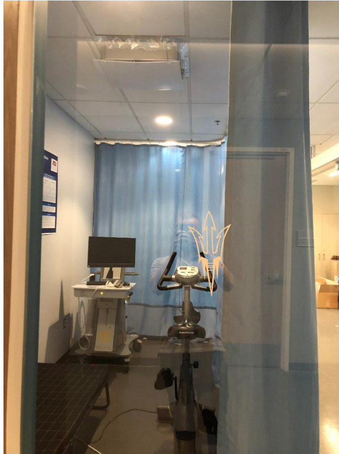
Figure 38. 4 th Smart Pad Operating Environment During Construction. Exercise bike, cot, and reference instrument all visible. Inlet fan (can be seen attached to ceiling) was totally sealed for all ambient VCO 2 assessments. Photo taken from outside the ambulatory area through a window visible from the hallway.
