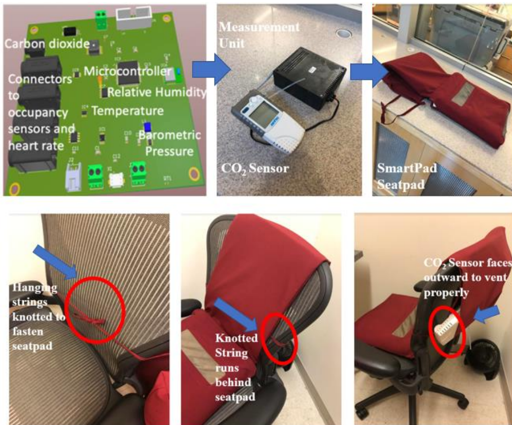
Figure 3: Smart Pad Hardware Components and Assembly Process. Measurement unit (houses sensor PCB shown in top left) and CO 2 sensor are fitted for Smart Pad seat cushion opening. The Smart Pad is tied around an office chair, where it is used to take EE measurements for the seated person.
