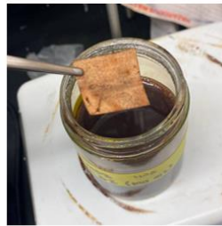
Figure 5.20 Physical mixing process for addition of DHPZ on commercial membranes with various concentrations.
