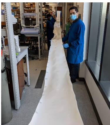
Figure 4.14 TFC membrane fabricated with automated draw down machine.
