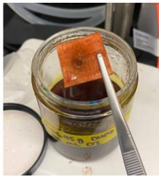
Figure 5.20 Physical mixing process for addition of DHPZ on commercial membranes with various concentrations.
