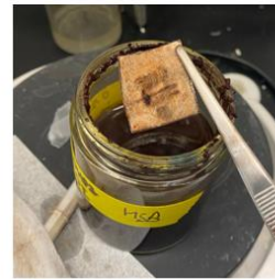
Figure 5.20 Physical mixing process for addition of DHPZ on commercial membranes with various concentrations.
