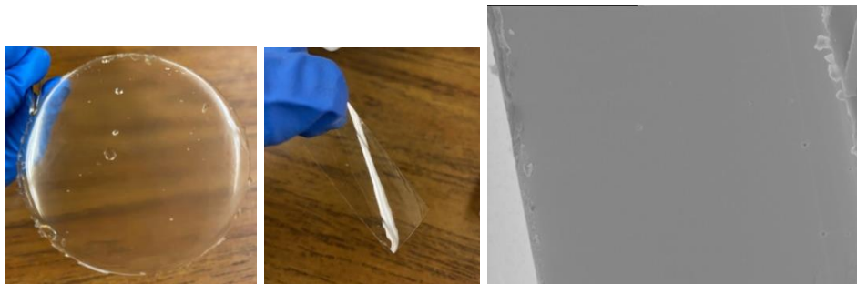
Figure 4.2 PSf membrane made following the dense membrane casting protocol (left and middle) and SEM image of the cross section (right).
