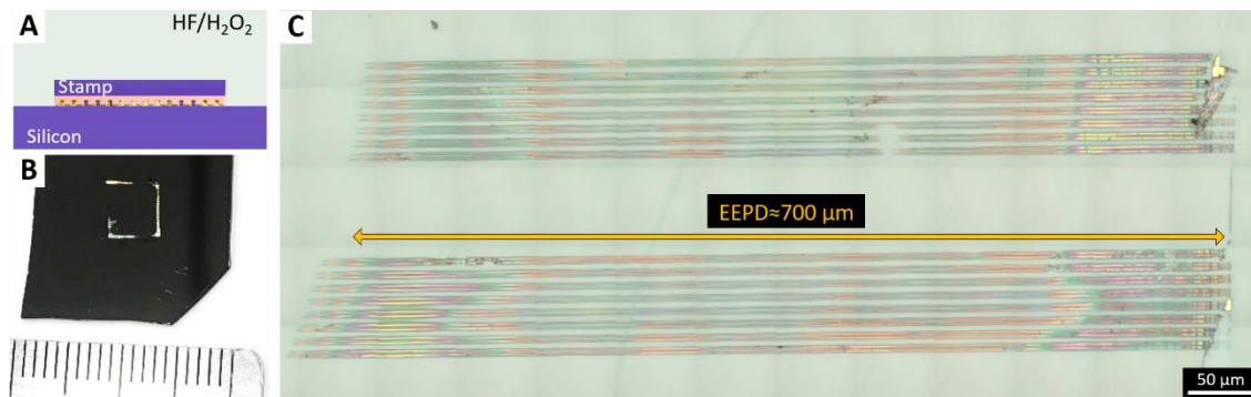
Figure 17. Analysis of the EEPD limitation. A – Schematics of the Mac-Imprint onto the blank SOI chip. B – Photograph of the Mac-Imprinted SOI chip. C – Optical image of the edge of imprinted area highlighting the EEPD.
