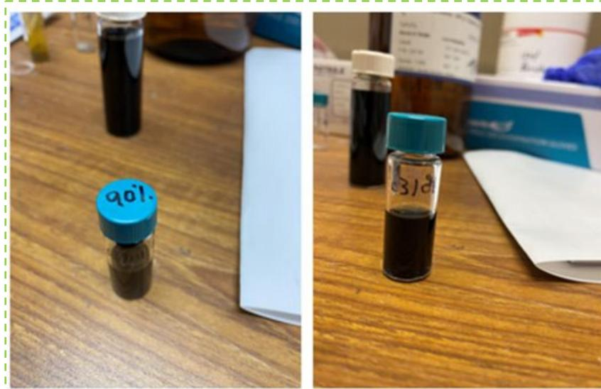
Fig.12 Prepared PEDOT:PSS solution. (10% PEDOT in 90% IPA v/v)
