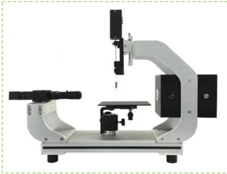
Fig.18 Contact Angle meter <sup>[59]</sup>.
