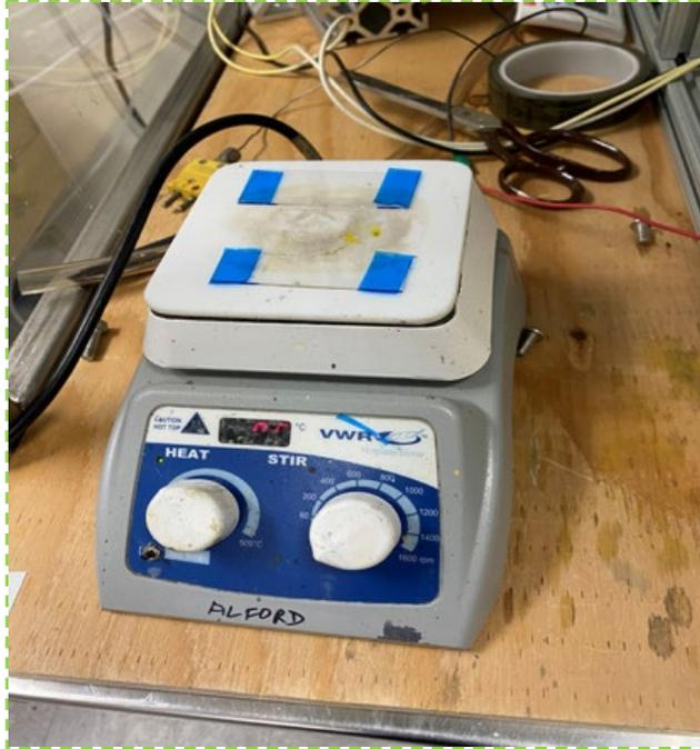
Fig.15 Printed ITO slides kept for annealing on ALT VWR Ceramic Stirrer.
