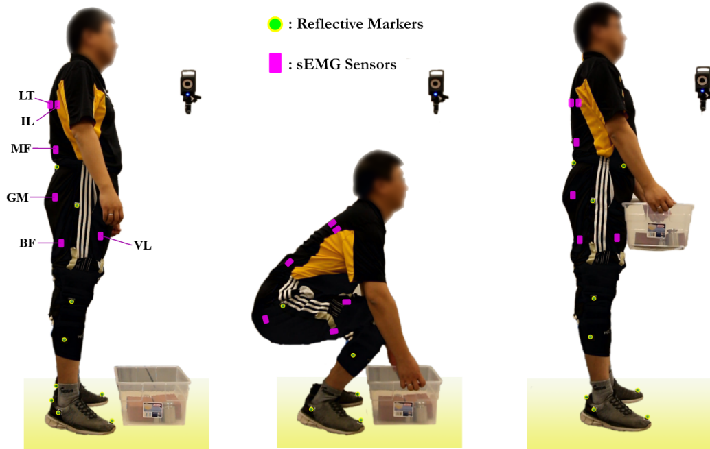
Figure 4.4. Human subject wearing the soft-inflatable exosuit and performing the lifting task. The abbreviations of the muscles investigated are depicted in the left picture. The EMG locations are approximated in the figure as these were placed underneath the clothing. The exosuit is inflated when the participant has reached the lowest position during the squat (middle picture) and assists through the upward lift.
