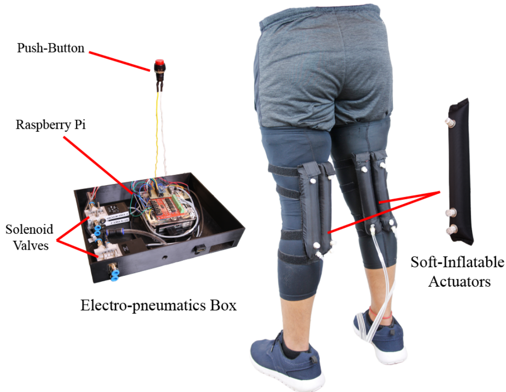
Figure 4.2. The soft-inflatable exosuit system worn by a human subject. The system is composed of two soft-inflatable actuators for each leg, solenoid valves, Raspberry Pi, and a push-button.
