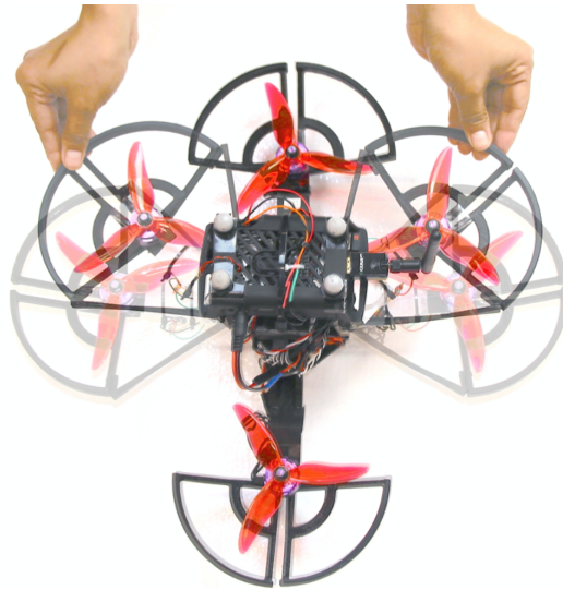
Figure 3. Morphing capability of SQUEEZE [6]
