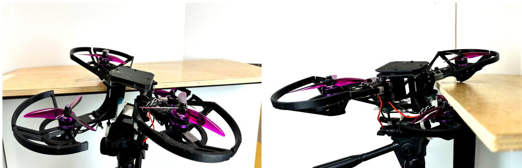
Figure 5. The adjacent propellers are off-axis which causes SQUEEZE to slide in and crash
