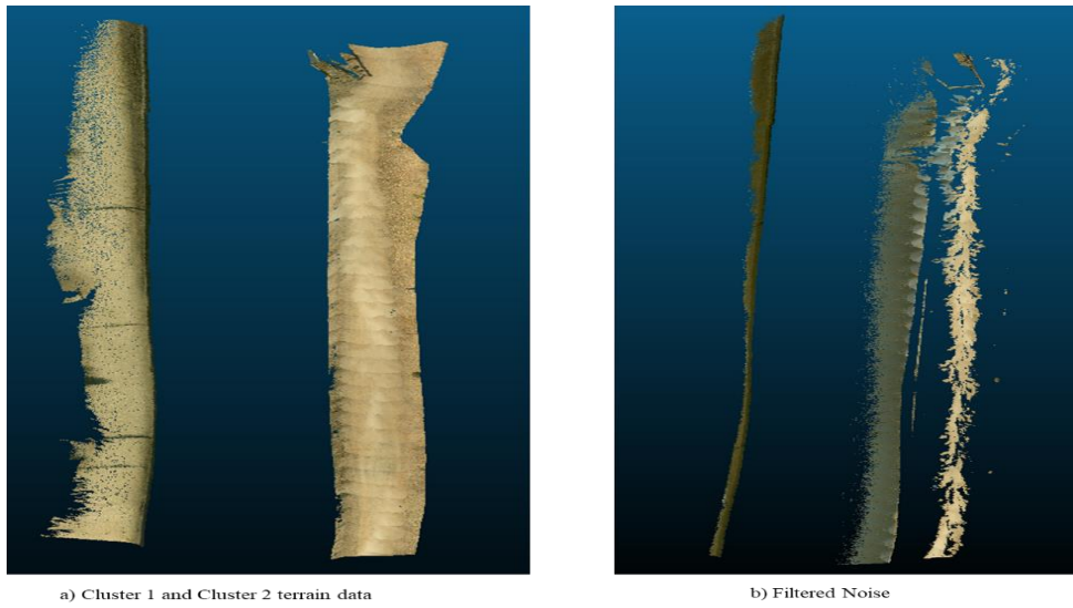
Figure 12. Processed Point Clouds Post-Noise Filter
