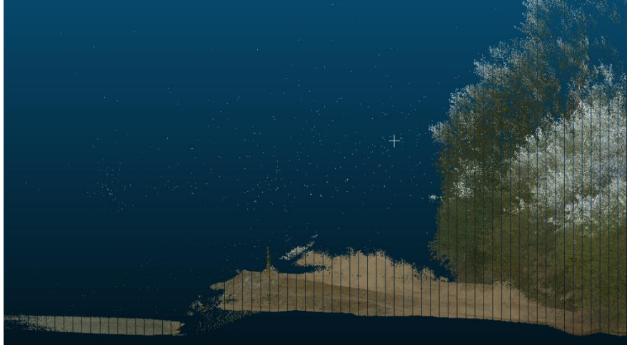
Figure 6. Noise in Raw Point Cloud Dataset
