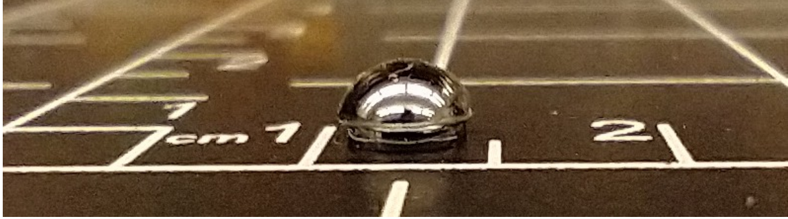
Figure 5.4: Side-view image of one prototype silicon lenslet with a single-layer glass AR cap/coating, with a \lambda/4 thickness centered at 150GHz.
