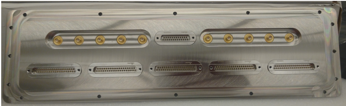
Figure 6.6: AliCPT VJ (300K) readout plate, the hermetic panel part of the readout harness design visible from outside the cryostat when fully installed.
