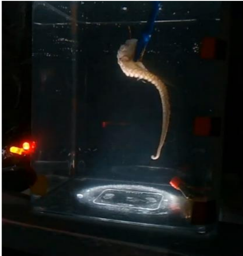
Fig. 7 In this figure, it shows more details for the experiment. For example, there is the red LED light at the corner to show the active status of the electrical stimulus input. Once the electrical stimulus stops, the LED light will be turned off. The LED can assist the authors to associate the EMG signals with the movements. In addition, the light under the container is to illuminate the experiment, or researchers cannot see anything in the video. Furthermore, this figure shows how the octopus arm bends during the electrical stimulus [29].
