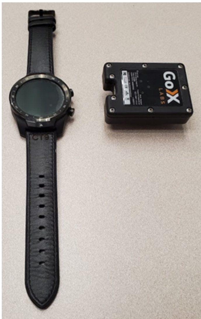
Figure 97: GoX Ergo Kit used in VO 2 and HR measurement. This is a similar device to what was used to test Airmen at Travis AFB in late 2019.
