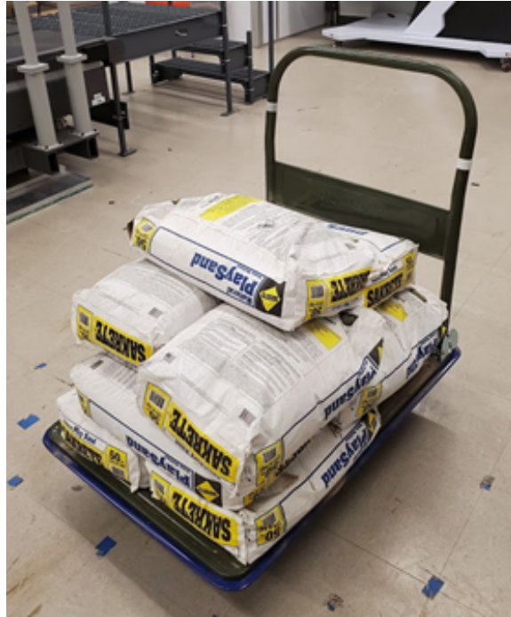
Figure 95: Testing equipment used for pushing. Five hundred pounds loaded on a cart. Future iteration will include a vertical wall for pushing against, as well as a containment system to contain errant weight material.
