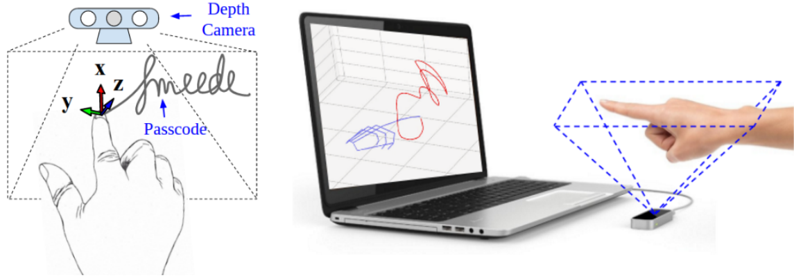
Figure 3.2: The Leap Motion Controller for Finger Motion Capturing
