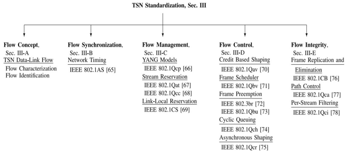
Fig 3 : Time Sensitive Networking (TSN) standardization [1]
