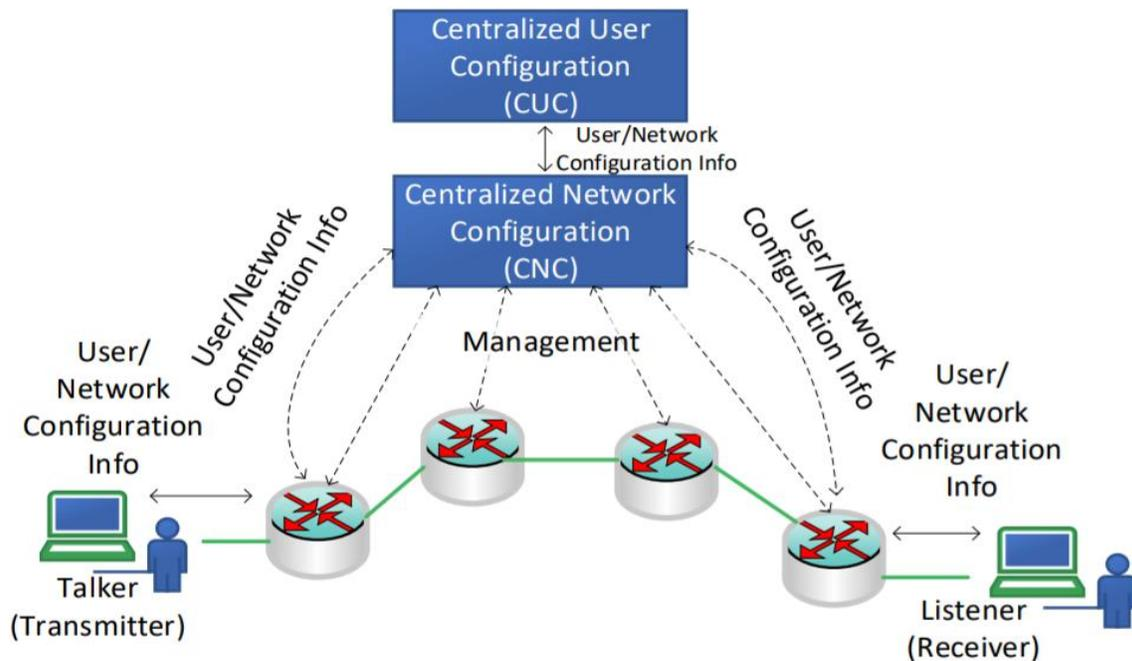
Fig 10 : Centralized Network Configuration (CNC) [19]
