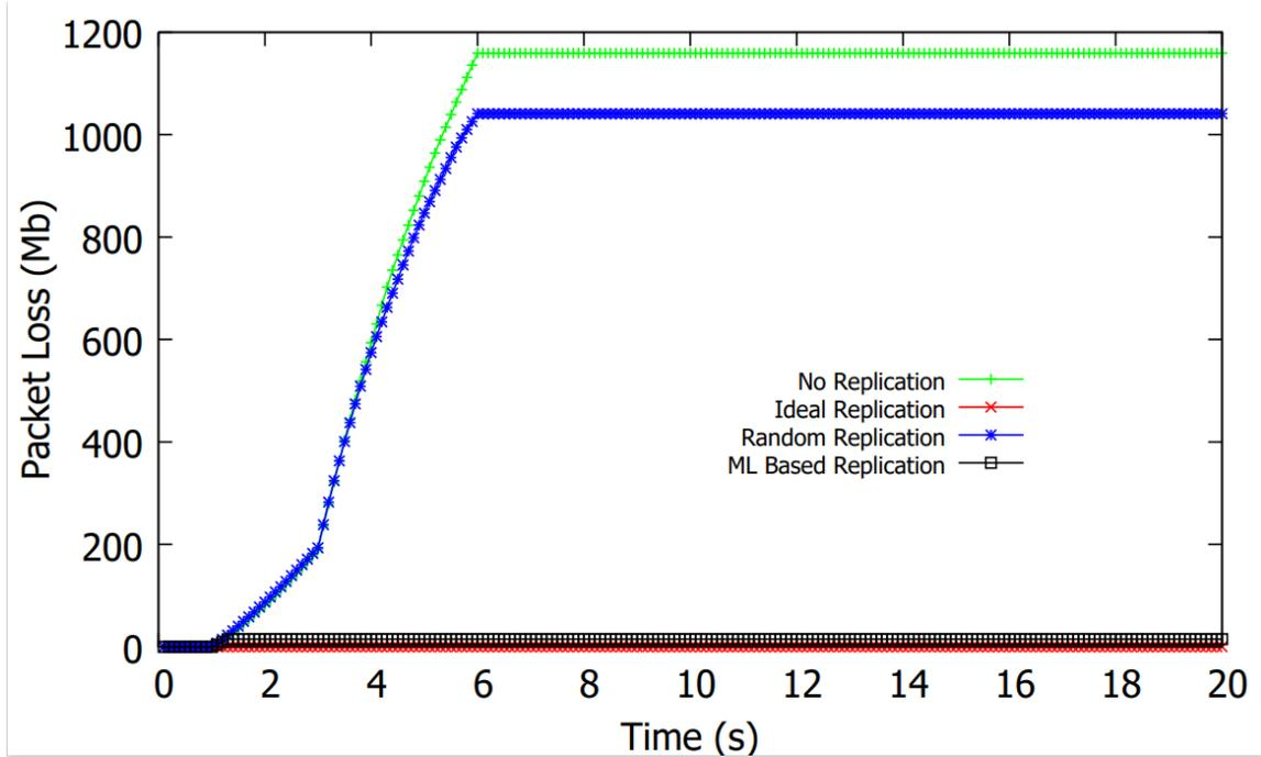
Fig 35 : Comparison of packet loss of each run type
