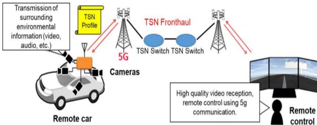
Fig 2 : Example of vehicular communication with TSN [26]
