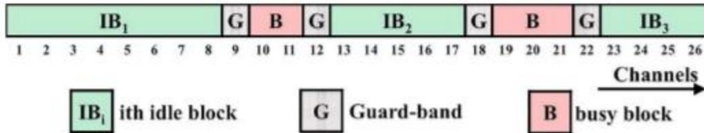
Fig 8 : Example of Guard Band [20]
