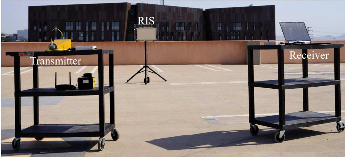
Figure: 3.15: The RIS-assisted wireless communication system consisting of an RIS, a transmitter (BS), and a receiver (UE). The transmitter and receiver are portable and can be placed in the far-field of the RIS surface.
