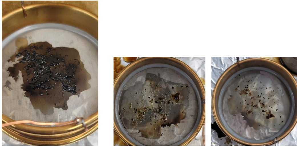
Figure 16- Fiber Distribution Within Diluted Asphalt Crack Sealant
