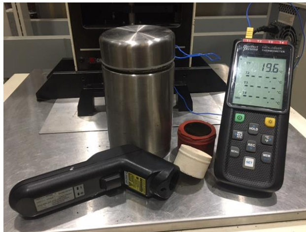
Figure 20- Specific Heat Capacity Testing Equipment
