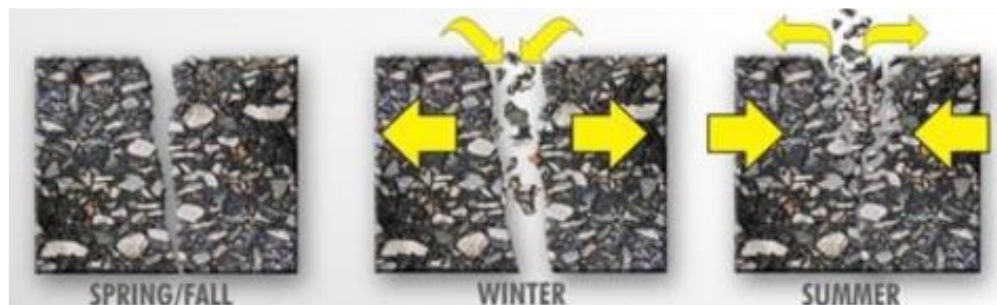
Figure 6- Intrusion of Incompressibles Damages in Cracks (For Construction Pros, 2017)
