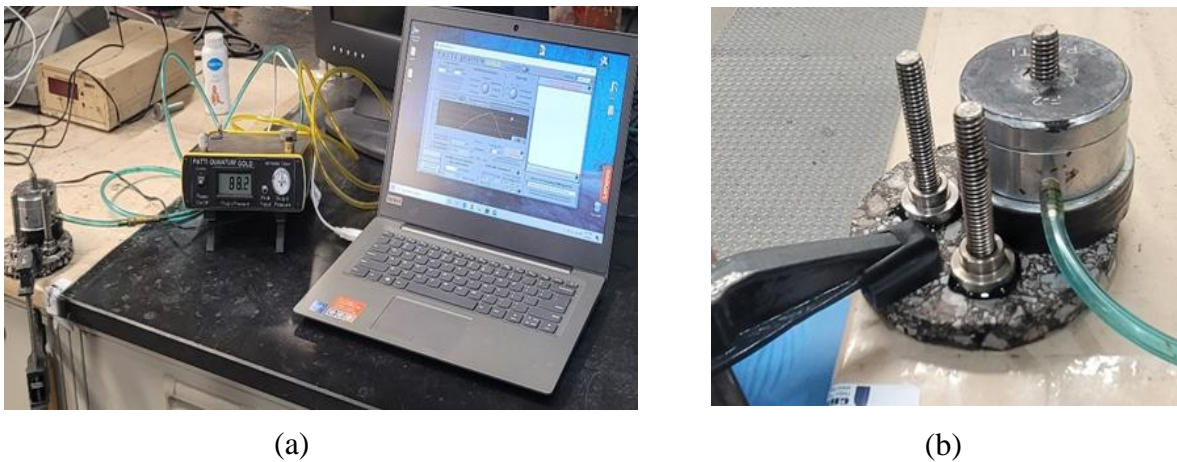
Figure 18- BBS Testing Equipment: (a) Type IV tester; (b) Stubs and Substrate Samples
