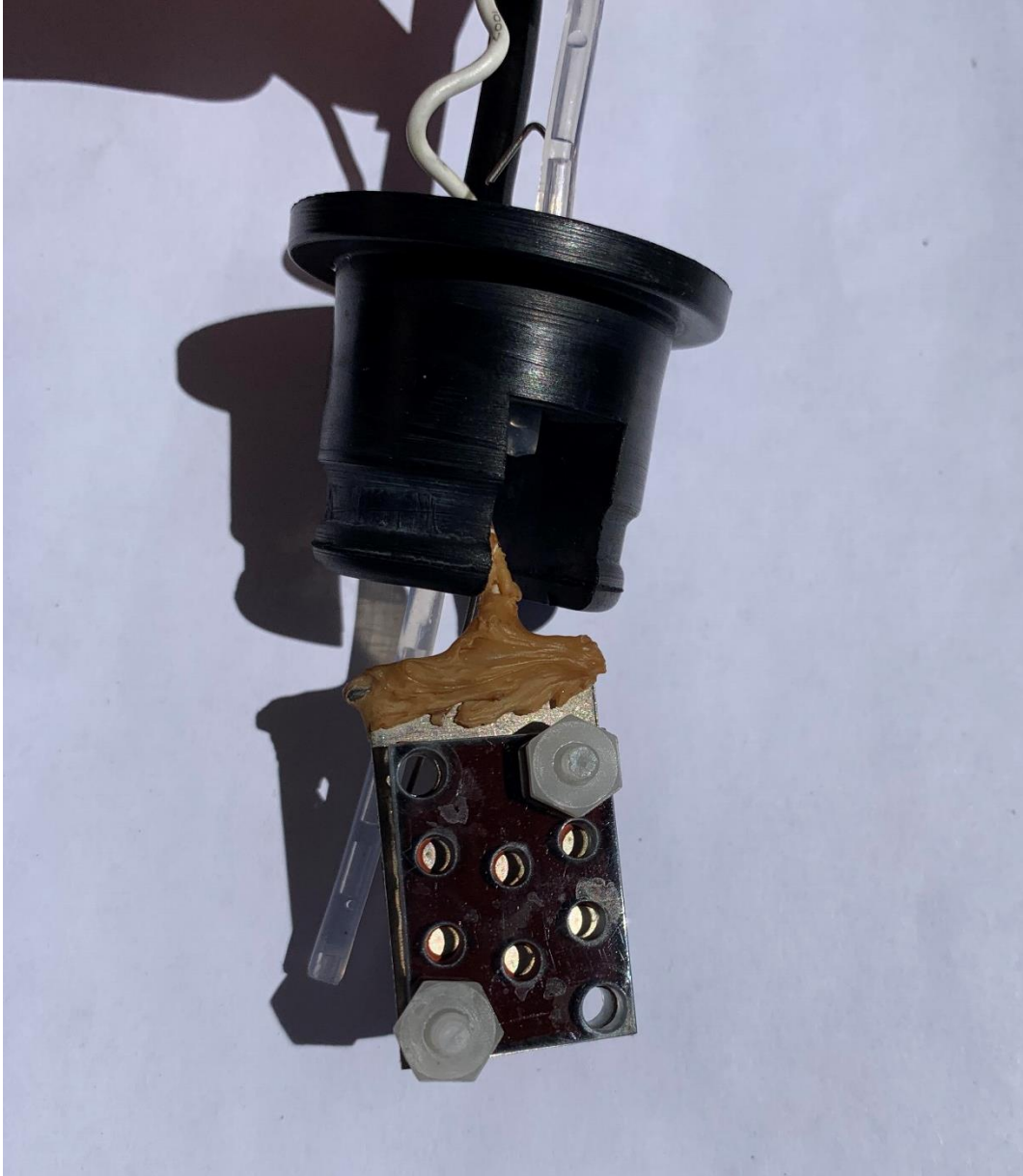
Figure A.9 Photograph of the grid holder used in a microbial electrochemical cell to grow G. sulfurreducens directly on EM grids for cryoET preparation.
