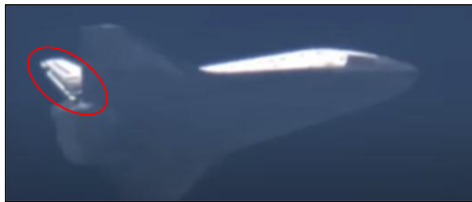
FIGURE 61. Elevator Up and Split Rudder “Speed Brake” Deployed at Mach 2.
