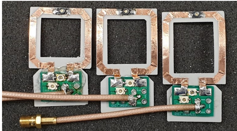
Figure 16. Ideal RF Coils Imitate 0%, 10%, and 20% Stretching Lengths
