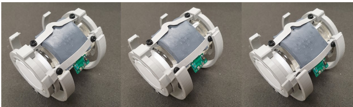
Figure 33. The Stretchable Dielectric Integrated RF Coil on the Stretcher
