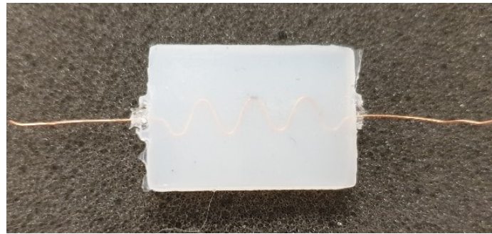
Figure 11. Elastically Stretchable Conductor
