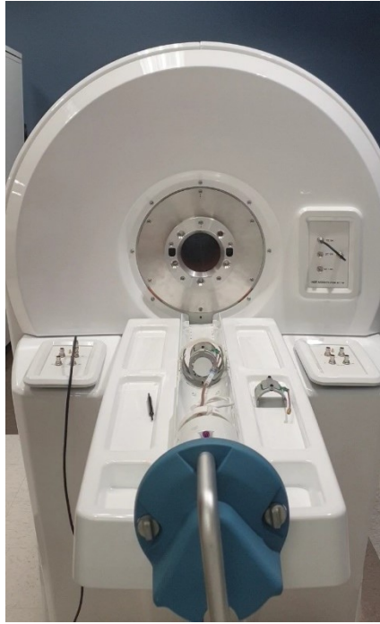
Figure 7. Dry Magnet MRI Scanner (9.4T)
