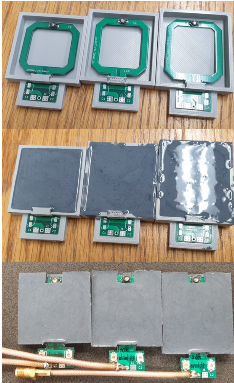
Figure 26. Dielectric Integrated Coils Fabrication Process
