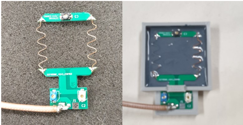
Figure 31. Stretchable RF Coil Fabrication Process
