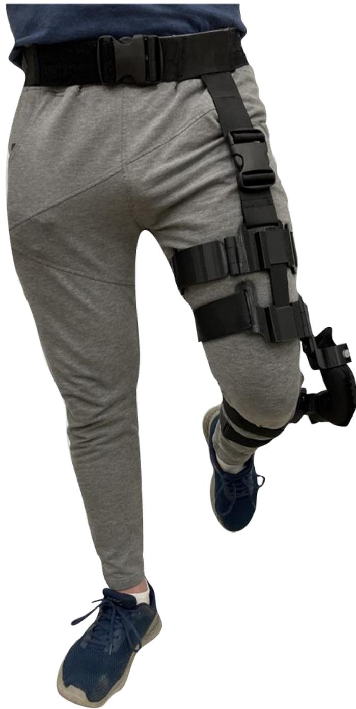
Figure 2.12. Front View of the Real Integration of the Exosuit in Inflated State.
