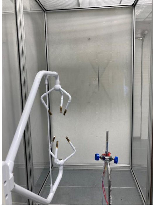
Figure 2.5. Picture of the typical experimental arrangement of the 3D ultrasonic anemometer side-by-side with the heated cylinder.
