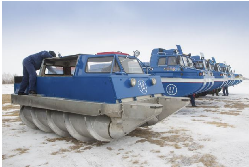
Figure 5. The ZIL-2906, a Screw-Propelled Russian Cosmonaut Recovery Vehicle.
