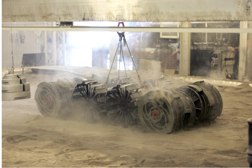
Figure 4. NASA RASSOR Bucket Drum Continuous Excavation Vehicle Operating in Lunar Regolith Simulant.
