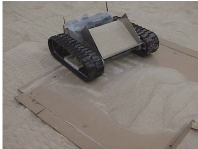
Figure 3. NASA Cratos Discrete Scraper Excavation Vehicle Depositing Lunar Regolith Simulant.
