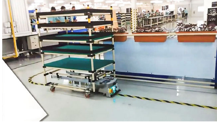
Figure 3.3: An Autonomous Guided Vehicle (AGV) Following a Path Laid Out in Tape
