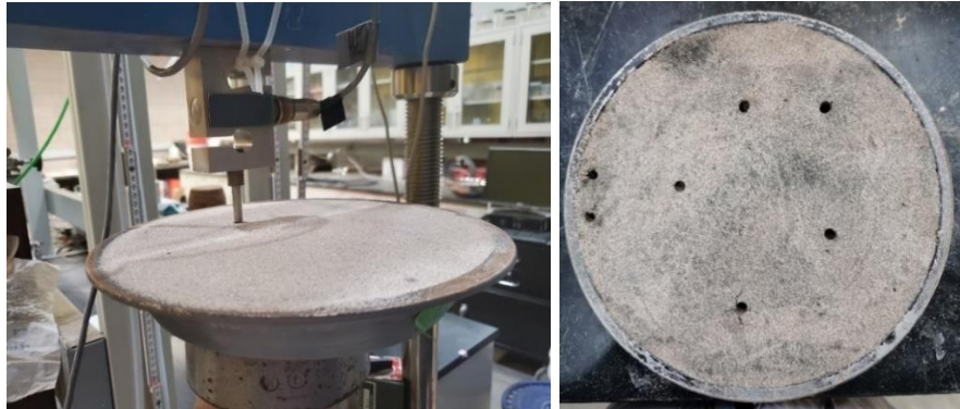
(a) (b) Figure 3. 1. a) Penetrometer Test on a Pan Specimen and B) Treated Sample after Performing Five Penetration Tests
