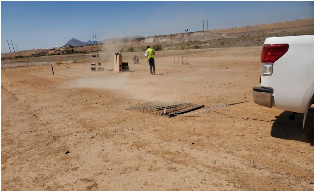
Figure 6. 6. Induced Dust Event Along the MICP Plot with the Truck Dragging a Chain Link Fence at Speed of 10 mph.
