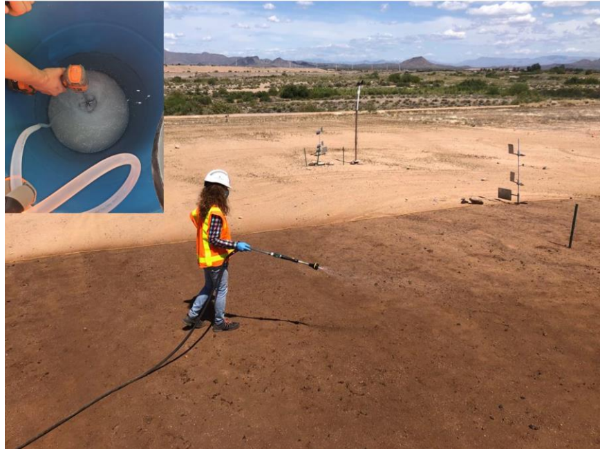
Figure 6. 4. Preparing the Cementation Solution and the MICP Treatment in Progress in SRL Field.
