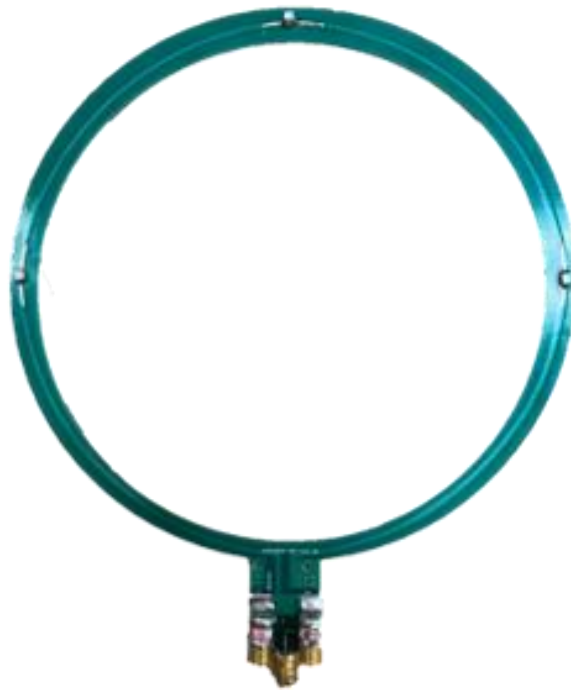
Figure. 16 PCB-based surface loop coil
