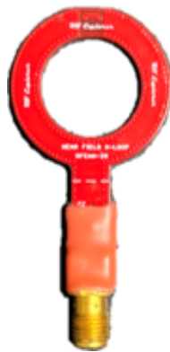
Figure. 7 RF Explorer H-field probe used for measuring transmission line noise
