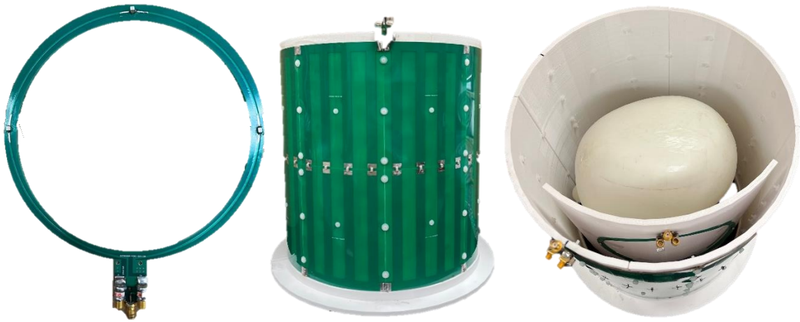
Figure. 29 PCB coils used in standalone STAR
