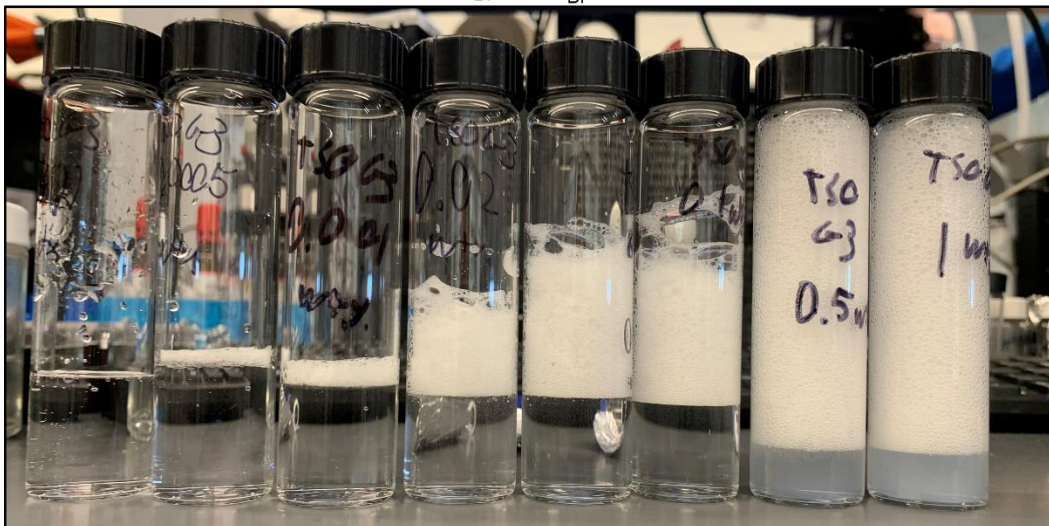
Figure 10.4. Trisiloxane cationic gemini surfactant formed stable foams upon agitation and the expansion ratio varied as a function of surfactant concentration.
