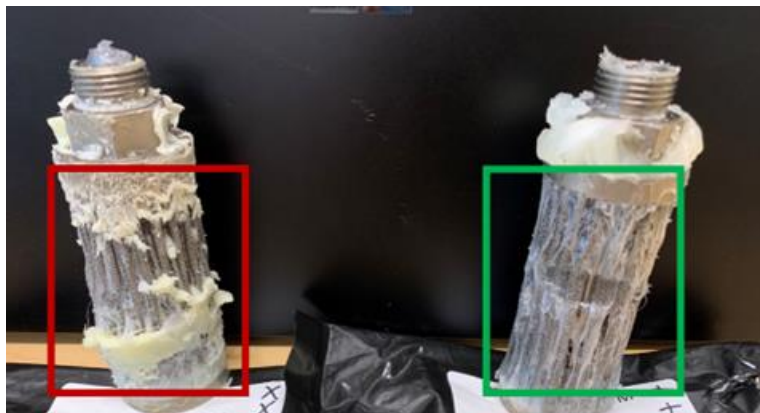
Figure 4.1. (Left) Example of solid white material building up on candle filters during extrusion and (Right) a clean candle filter without any extrudate buildup.
