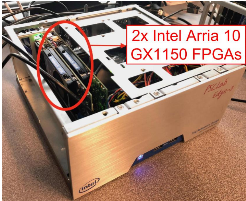
Figure 3.1: An Intel Fog Reference Design Unit Hosting Two Nallatech 385A FPGA Acceleration Cards.
