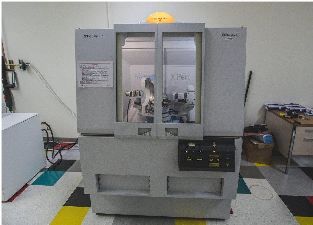
Figure 4: PANalytical Xpert Pro XRD Machine. [22]
