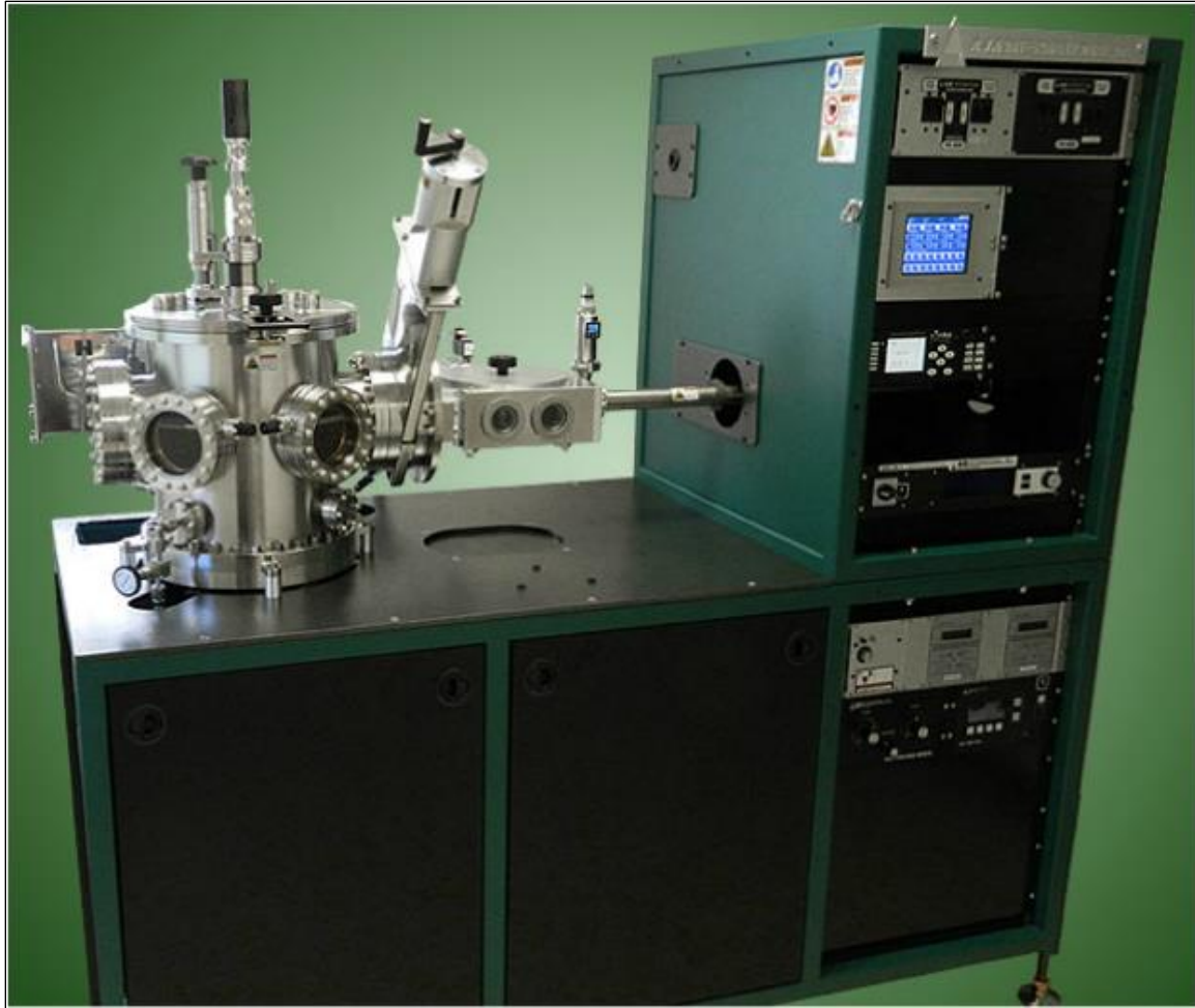
Figure 3: AJA Orion-5 Magnetron Sputtering System. [12]
