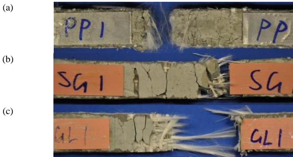
Figure 3.38 Distribution of cracks on the tested samples: (a) PP, (b) SG, (c) GL
