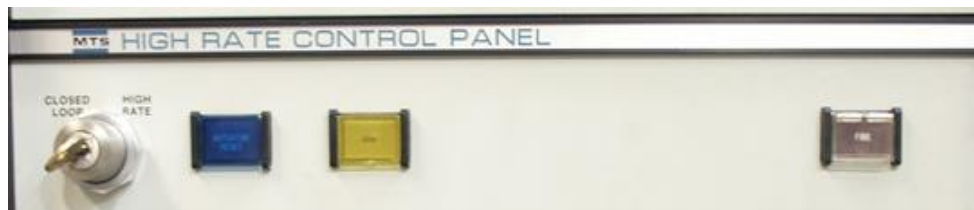
Figure 1.6 High Rate Control Panel
