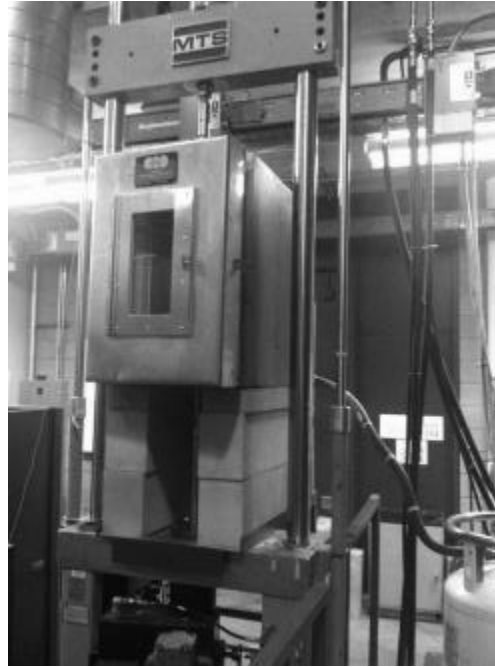
Figure 3.1 High speed testing machine with environmental chamber at Arizona State University
