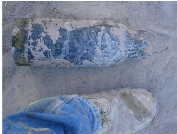
Figure 5.4 Broken HDPE Pipe from Drive Six
