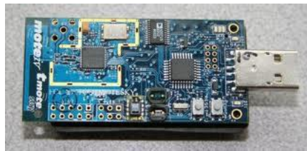
Figure 2 Telos revision B with sensors on board
