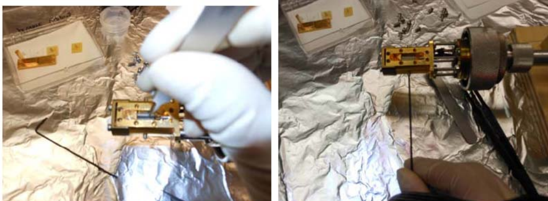
Figure B.4 loading the sample between fiber glass clamps and on top of the L-
