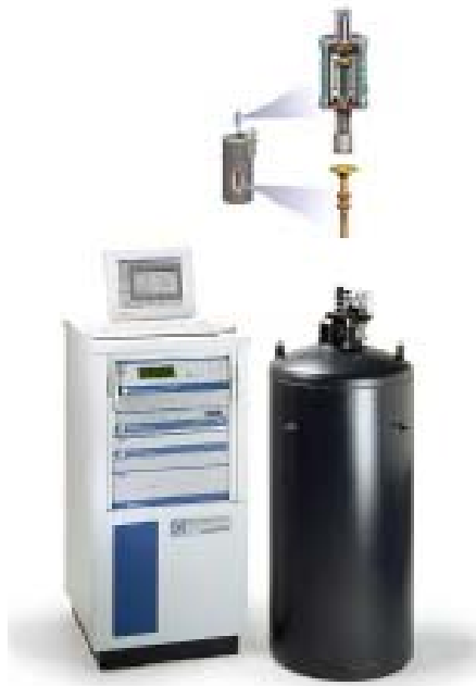
Figure B.2 Cryogenic systems: Necktube liquid helium dewar (left) and PPMS system (right)
