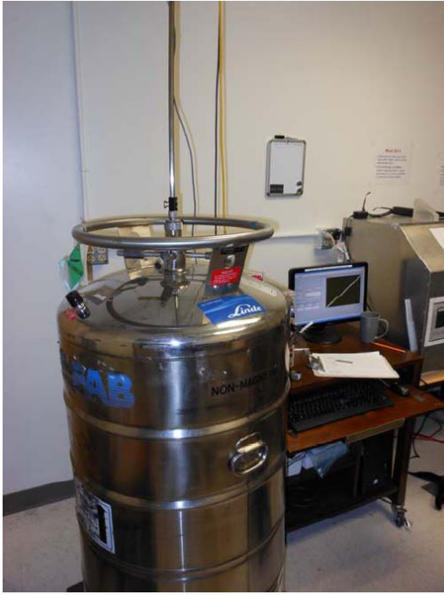
Figure B.2 Cryogenic systems: Necktube liquid helium dewar (left) and PPMS system (right)
