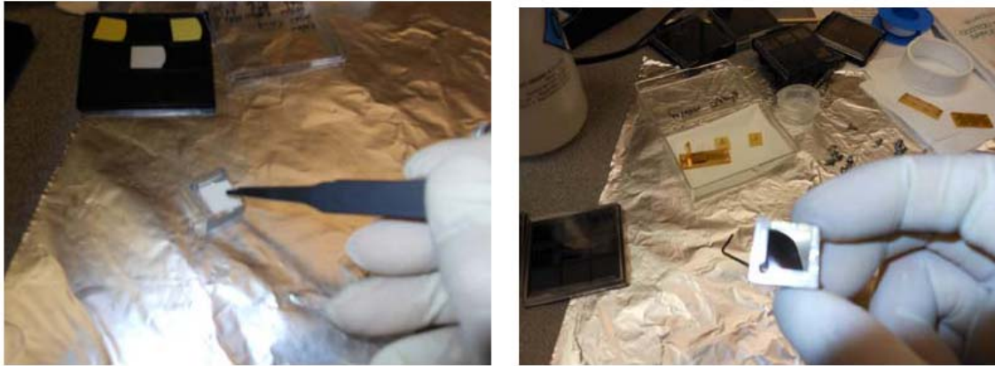
Figure B.3 loading the dielectric and superconducting films using the Aluminum square sample holder
