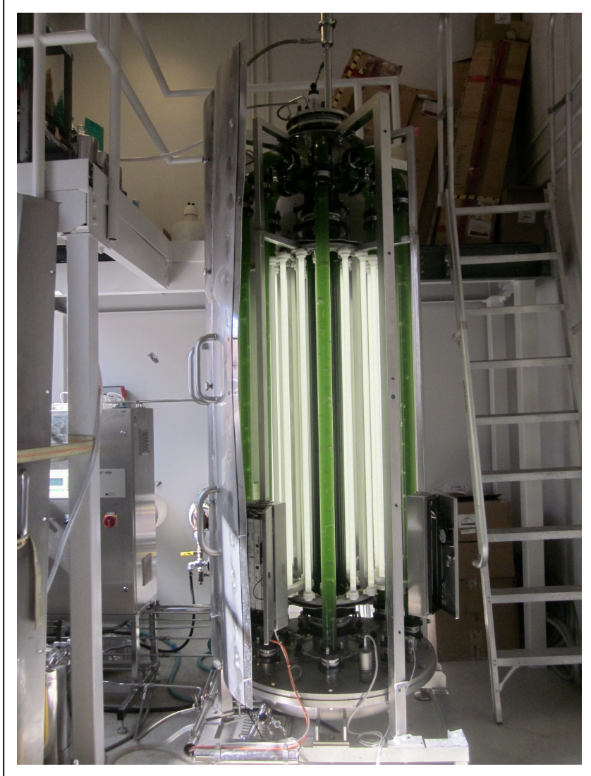
Figure 4.2. The bioreactor used to grow the thermophilic cyanobacteria, T. elongatus , which holds approximately 120 L of cell culture. The cells are grown at 56°C.
