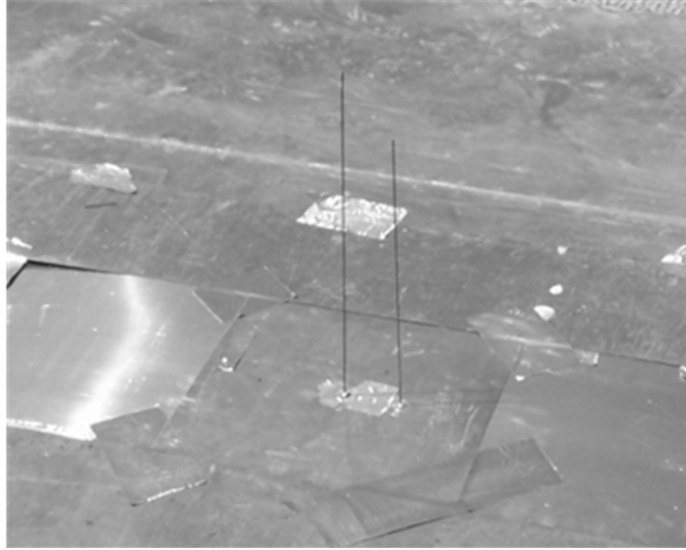
Figure 19. Two-port monopole fabricated to measure the S parameters and validate the MININEC calculations used in the theoretical study.
