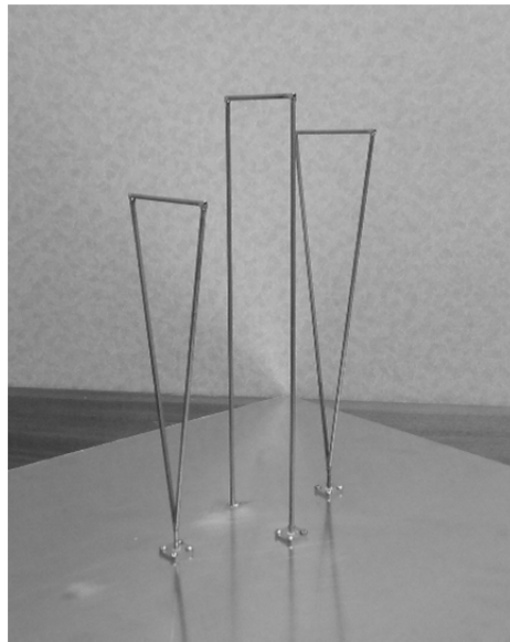
Figure 56. Fabricated compact Yagi–Uda antenna.
