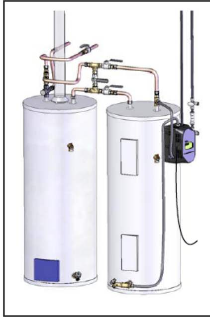
Figure 8. FAFCO® 500 Dual Tank Setup [12].
