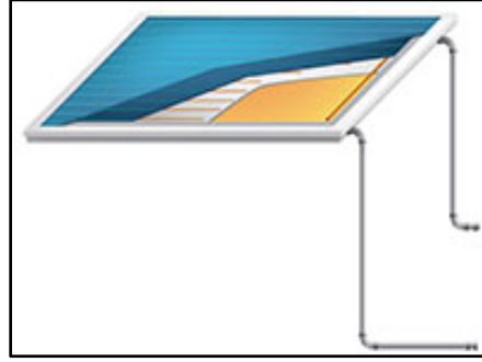
Figure 4. Glazed Flat-Plate Solar Collector [5].
