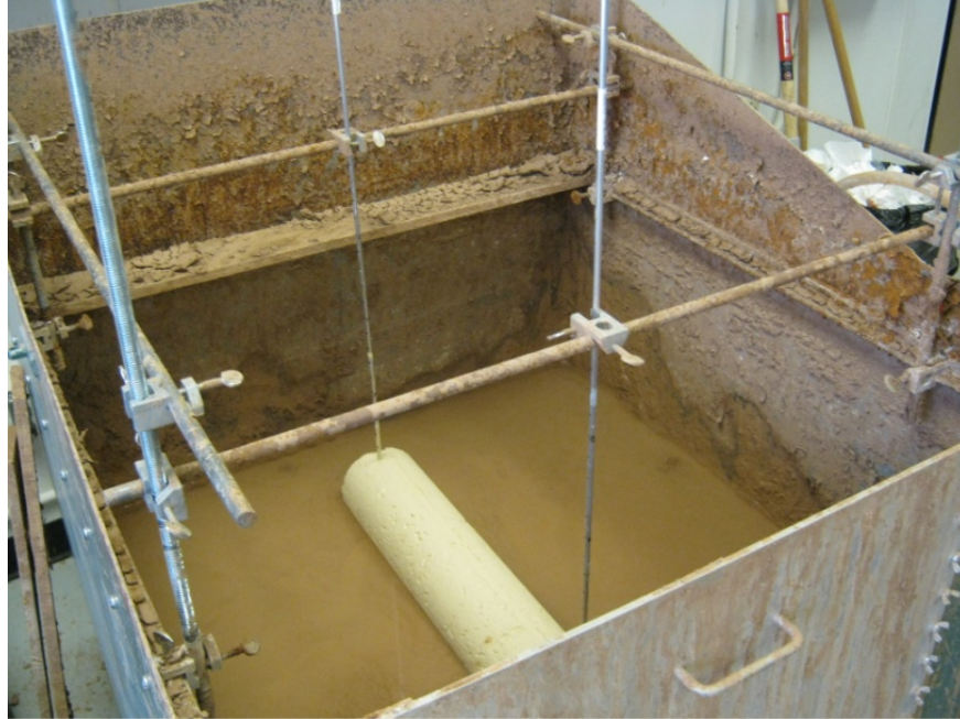
Figure 3.14 Experimental Setup for HDD
