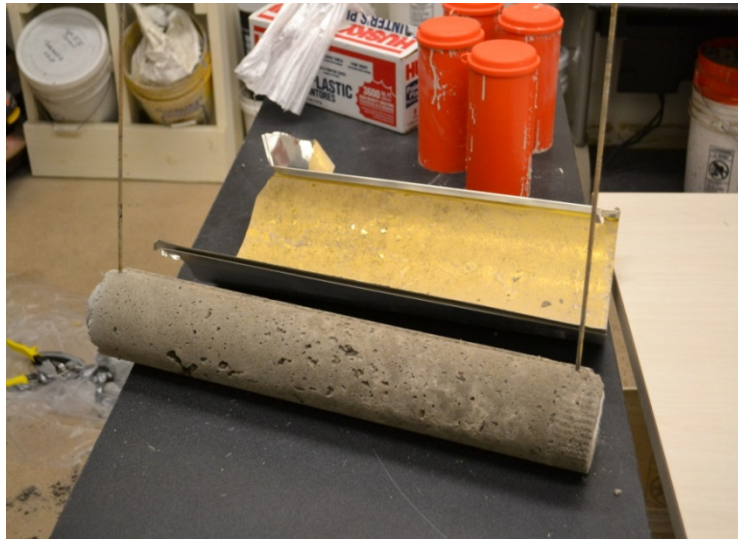
Figure 3.1 Light Concrete Mold for a HDD Pipe Assembly
