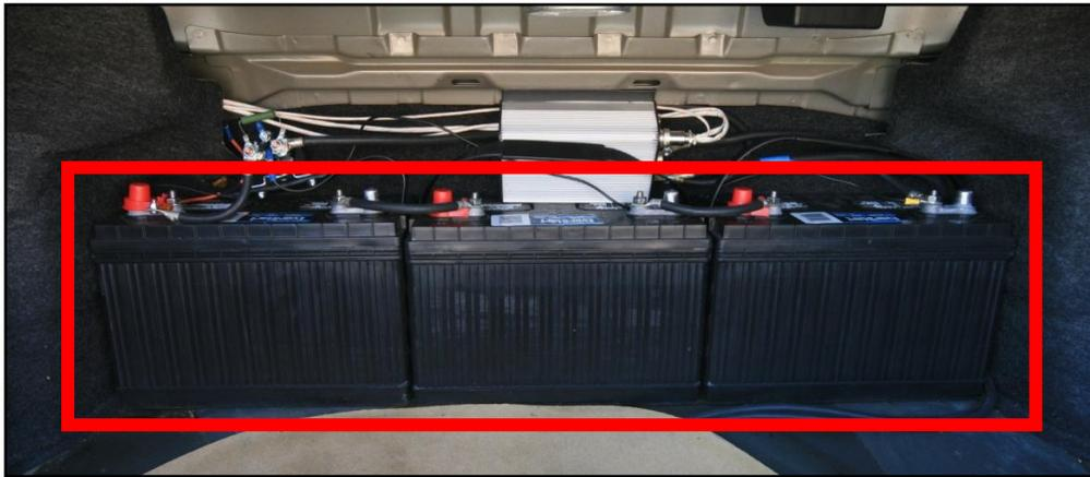
Figure 10. The 36 V EverStart® MAXX battery bank (trunk carpet removed).
