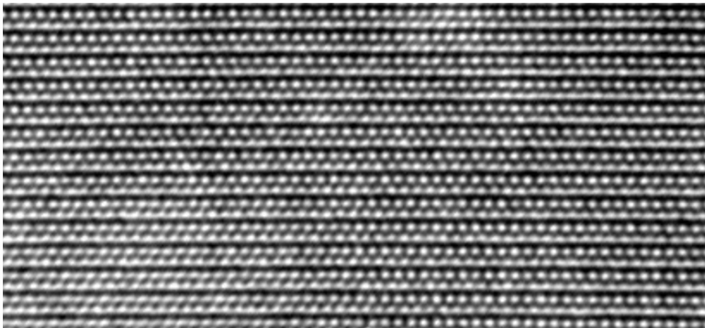
Fig. 2.6. HRTEM image of GaN along the [11\bar{2}0] zone axis. The atomic configuration matches well with the ball-and-stick model in Fig. 2.5.
