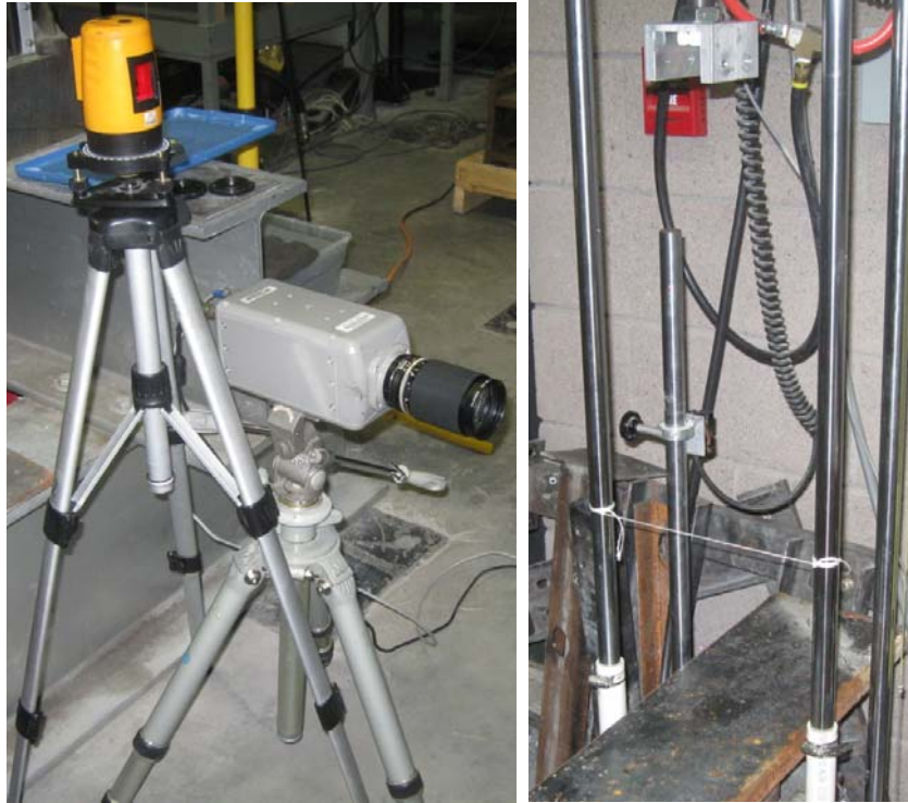
Figure 3-14: (a) Camera and laser level set-up; (b) testing machine and reference string
