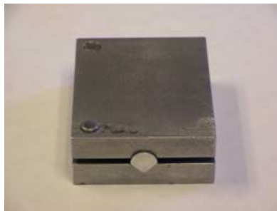
Figure 3-5: Specimen Gripping System for GN 2118
