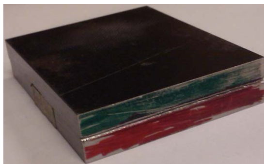
Figure 3-6: Specimen Gripping System for AS299
