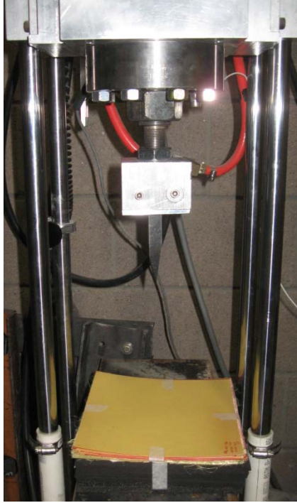
Figure 3-21: Sample set-up before testing with energy level 1
