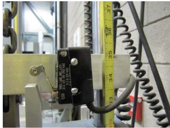
(a) (b) Figure 3-18: (a) Height control mechanism, (b) Release mechanism
