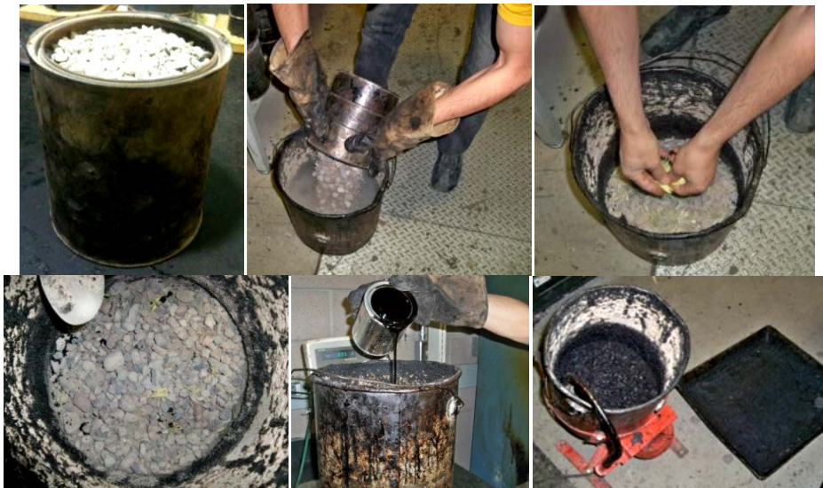
FIGURE 2 The HMA mixture process: (top left to bottom right) batched heated aggregates, pouring in mixing buckets, adding distributing pre-weighted fibers, mixing fibers and aggregates, adding binder, final HMA mixture.
