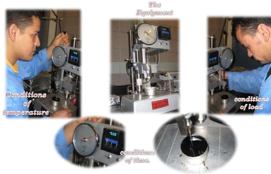
FIGURE 7 The penetration test steps.
