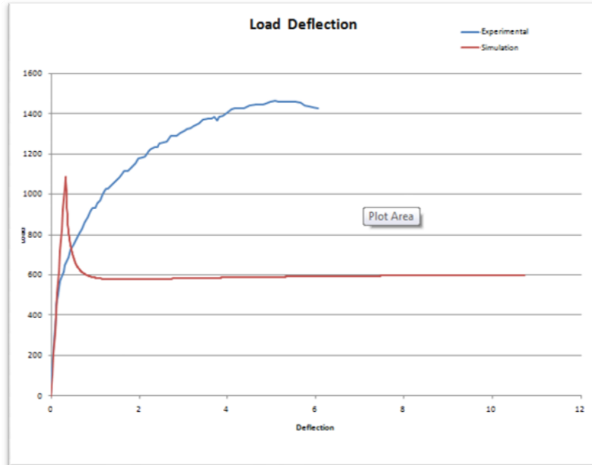
Figure A.2.1.2 – Linear section of load deflection clearly modeled by E=25000 MPa.
