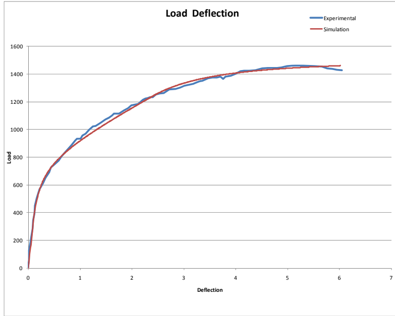
Figure A.2.1.7- Load deflection curve response to change in \beta_{tu} .
