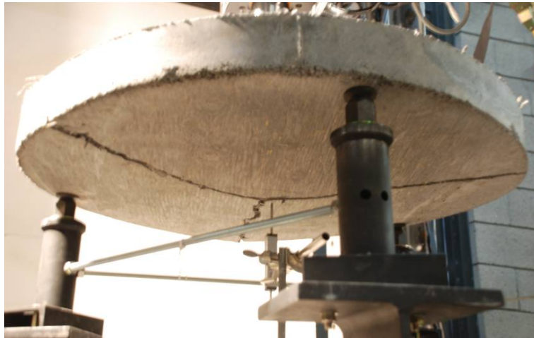
Figure 6.2.4 RDP with three concentric radial cracks at approximately 120 degrees.
