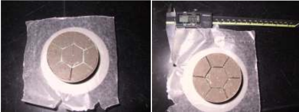
Figure 4.25. An example of different stages of creating a cracked specimen for SWCC tests
