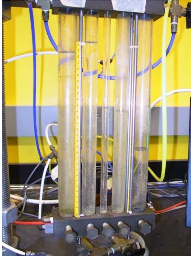
Figure 4.8. Illustration of removing the entrapped air from the system and filling the Volume Change Device (VCD) tubes
