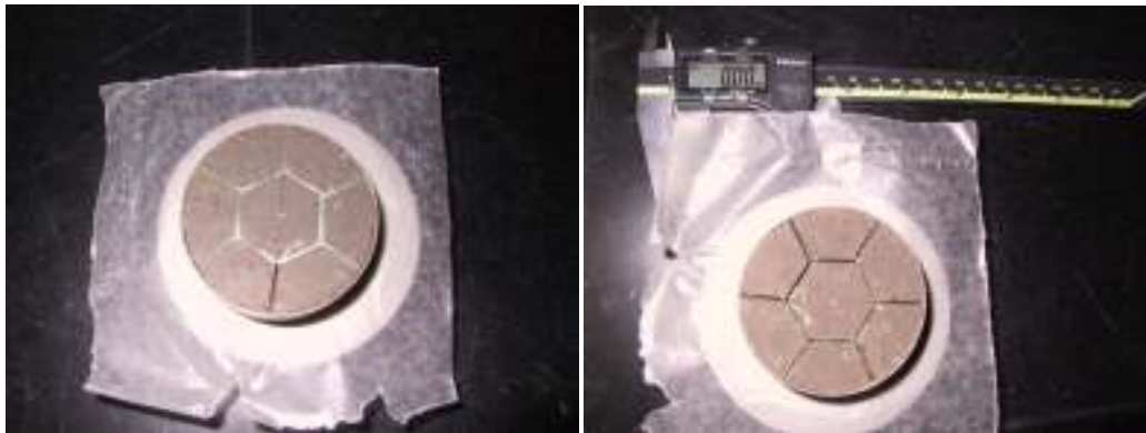
Figure 3.7. An example of different stages of creating a cracked specimen
