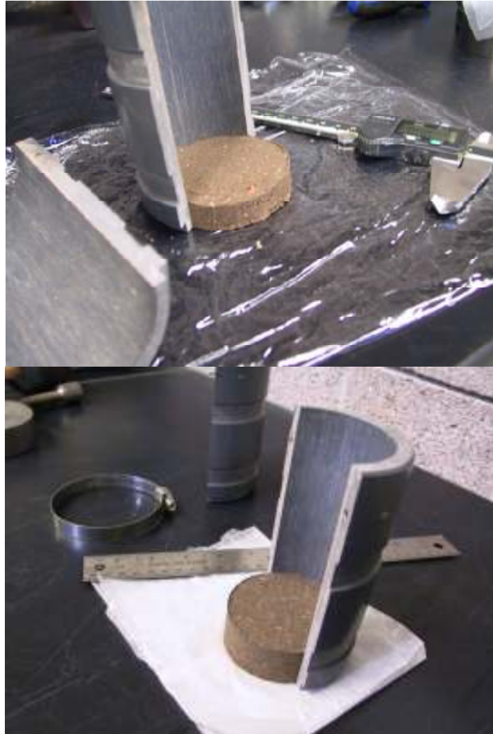
Figure 4.7. Illustration of different stages of sample preparation for direct k_{sat} measurement test
