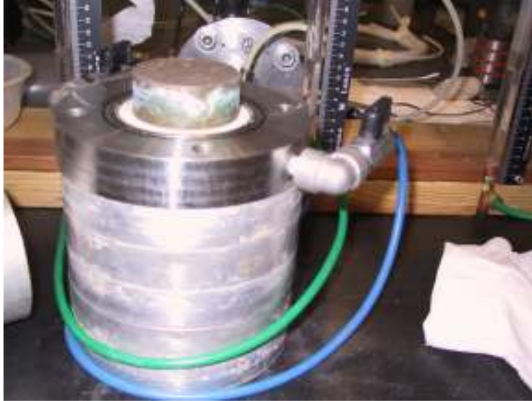
Figure 4.26. Illustration of hanging manometer technique for determination of SWCC for cracked soil
