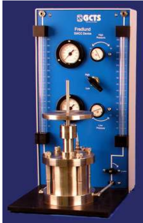
Figure 4.20. General view of Fredlund SWCC device (from www.gcts.com )
