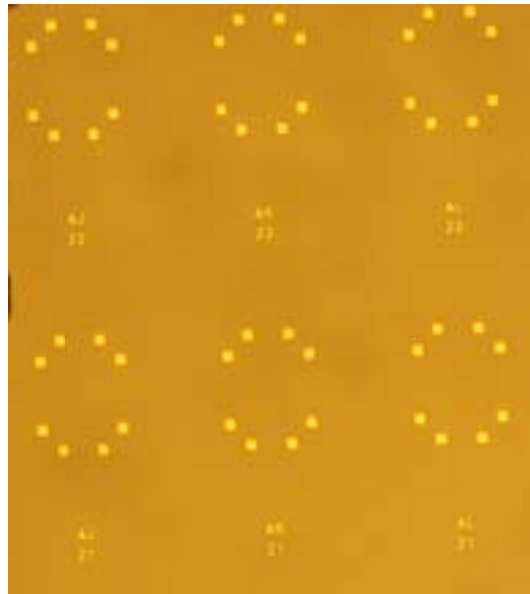
Figure 3.5 the gold alignment marker done by photolithograph. The row is marked by number and the column is marked by letters.
