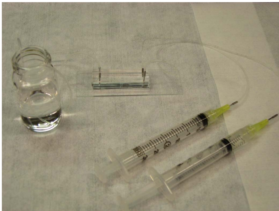
Figure 3.12 PDMS microfluidic delivery device.
