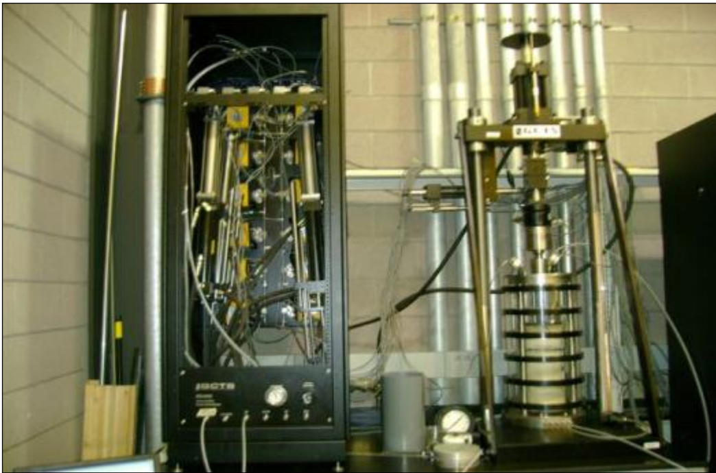
FIGURE 4-1 Special triaxial unit used for testing of saturated specimens
