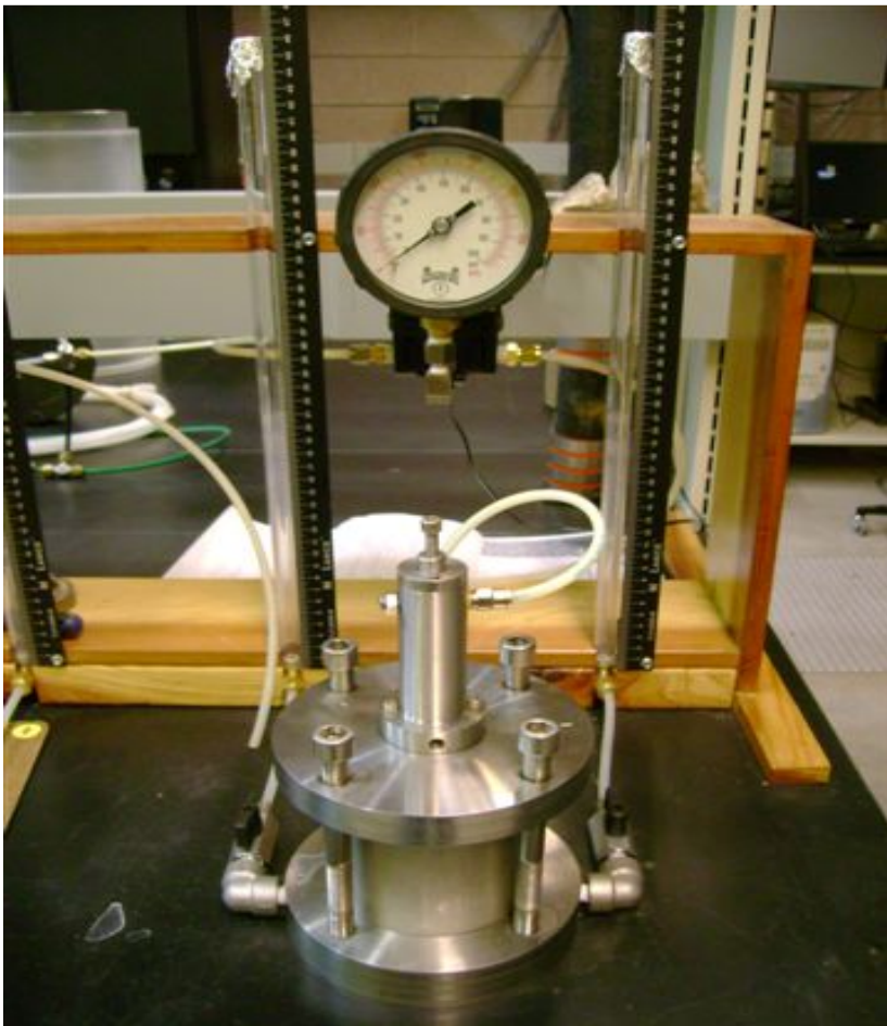
FIGURE 3-5 Pressure plate setup to obtain the SWCC of the soil
