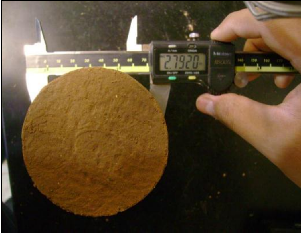
FIGURE 5-5 Measurement of specimen diameter after compaction
