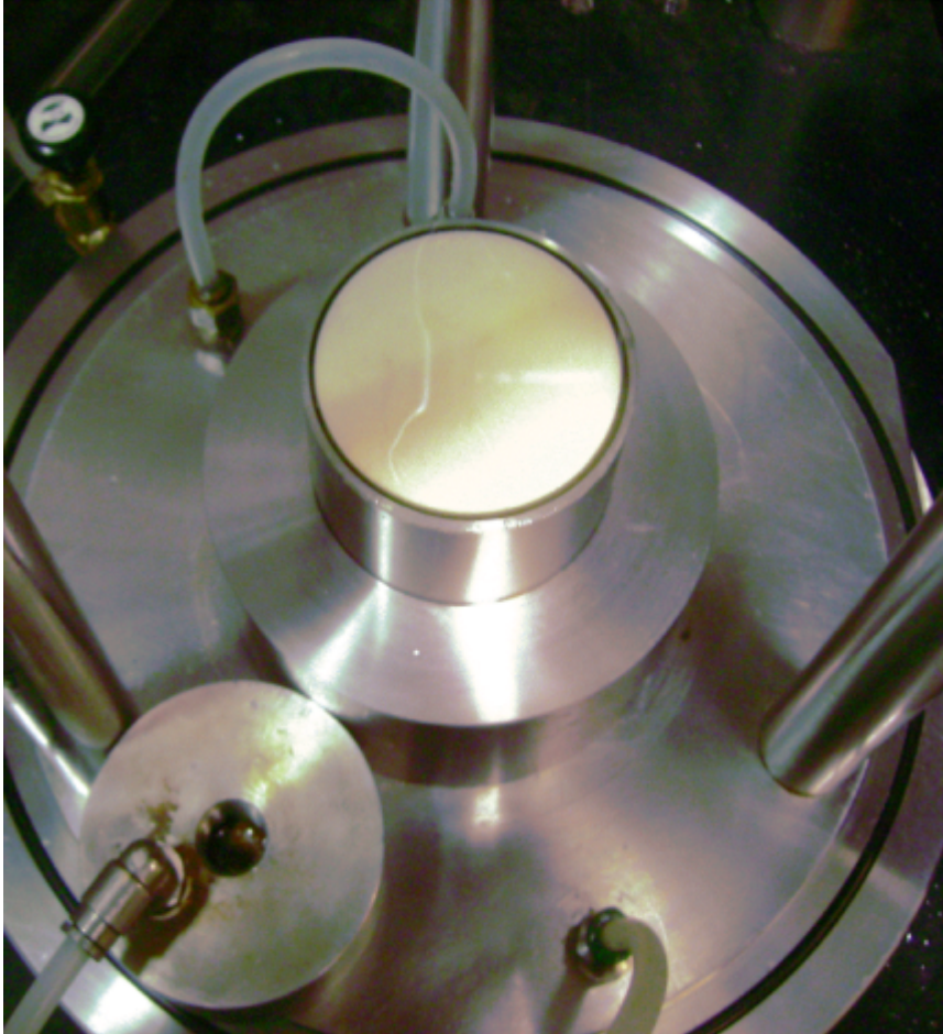
FIGURE 4-7 New bottom pedestal used for unsaturated testing
