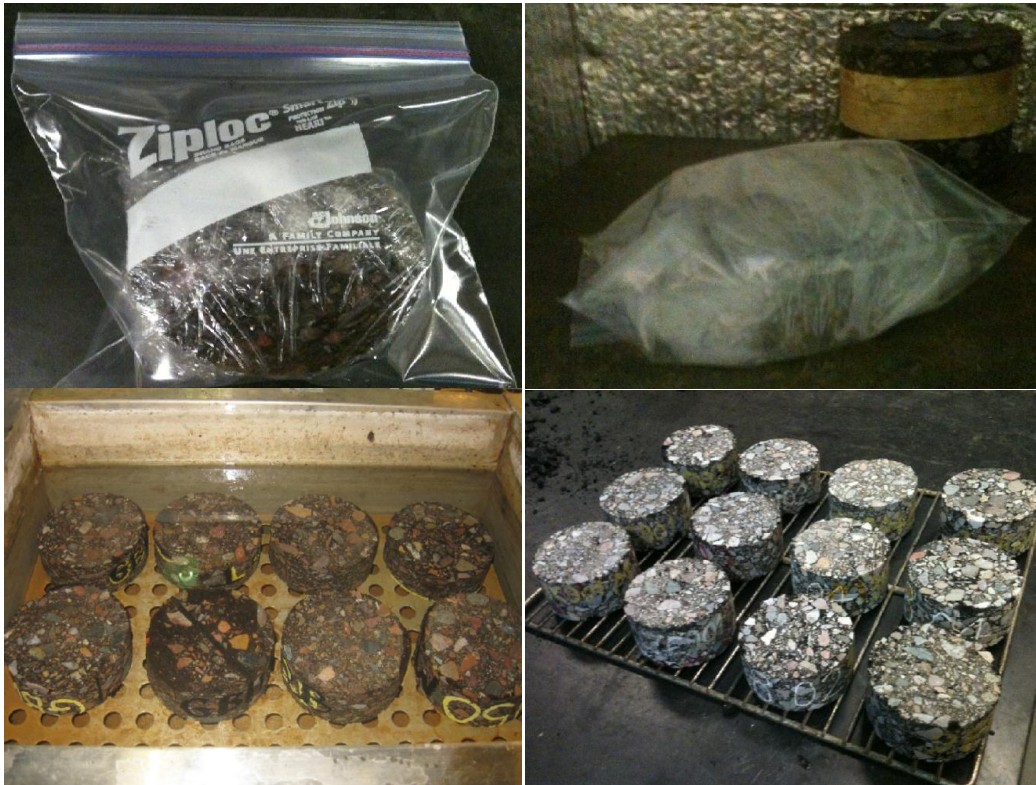
FIGURE 4 Freezing and thawing cycle.
