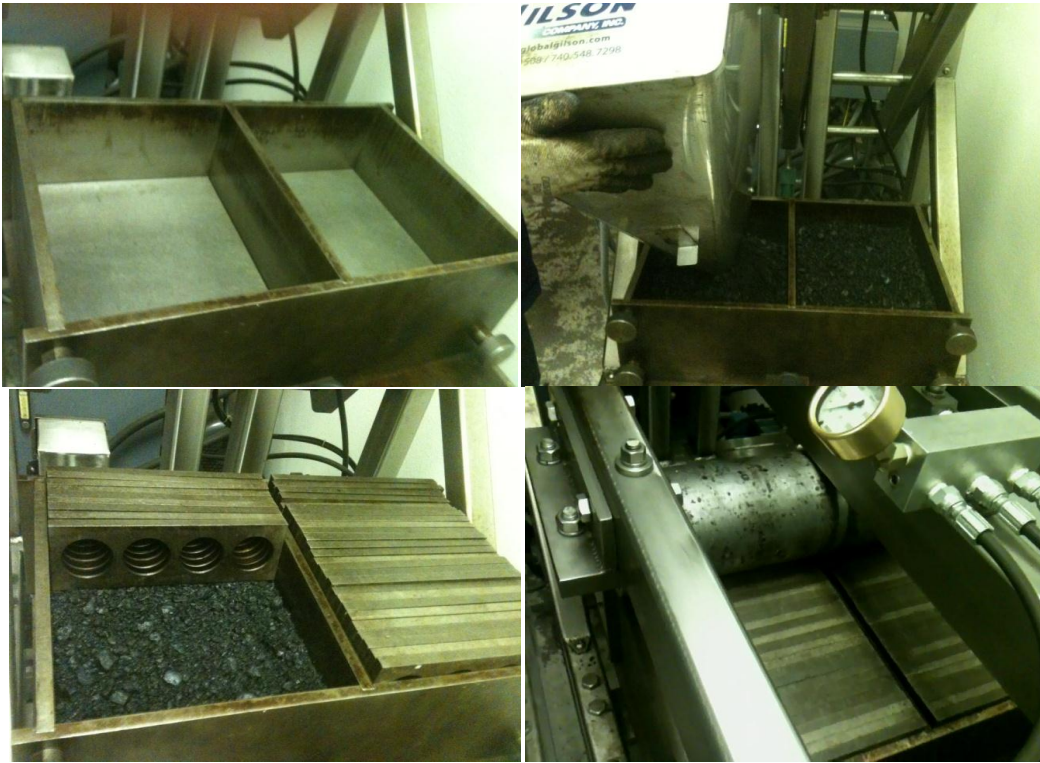
FIGURE 13 Compaction of beams using kneading compactor.
