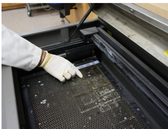
Fig 3.2: Laser Machine (Universal laser system) used for cutting glasses and making the coating cross sections
