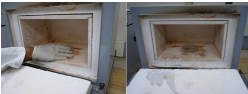
Fig 3.7: Sintering of electrodes in the furnace at 400\text{ }^\circ\text{C}
