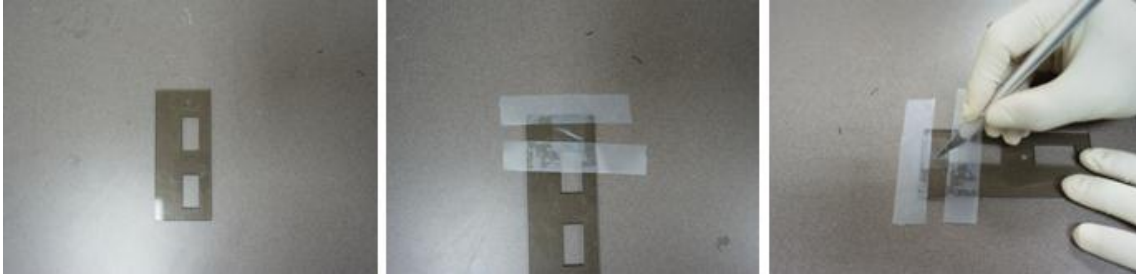
Fig 3.15: Modified Sealant cutting process
