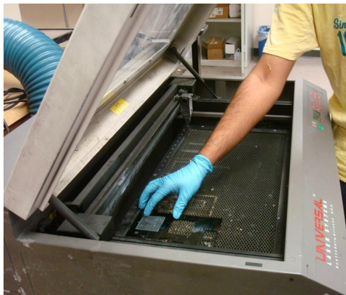
Fig 3.14: Cutting of glass electrodes using Laser (Universal Laser system)
