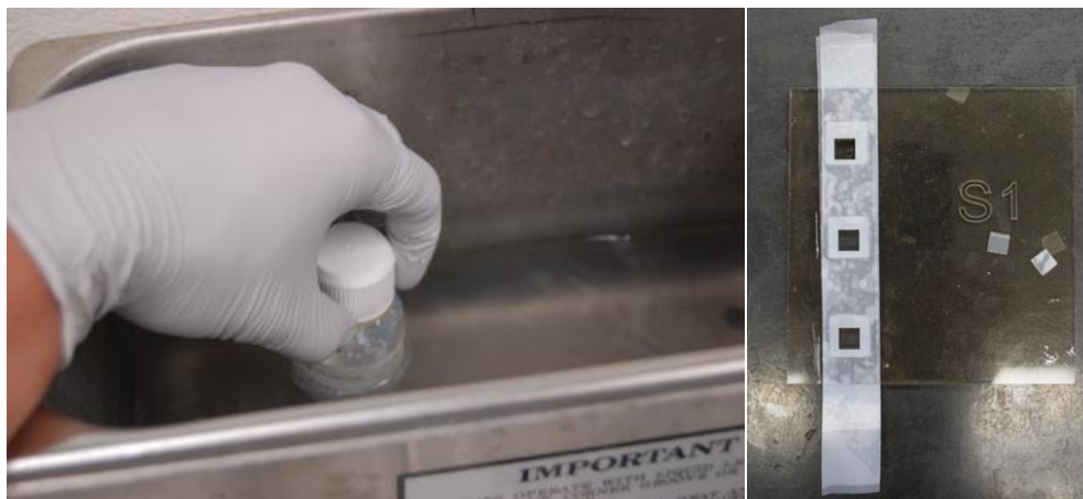
Fig 3.4: Sonication of \text{TiO}_2 paste and cell area definition on substrate using scotch tape
