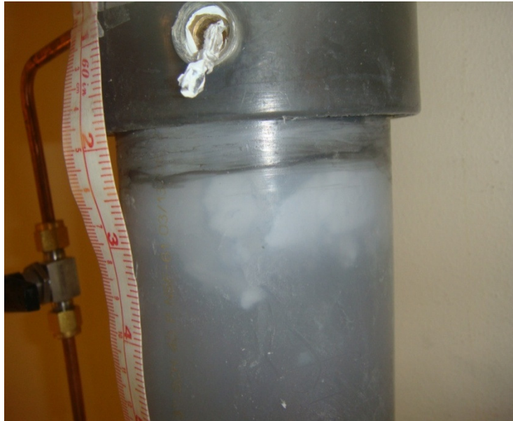
Figure 6-33. Photo showing severe particle agglomeration with fluidizing fine Nanogel particles.
