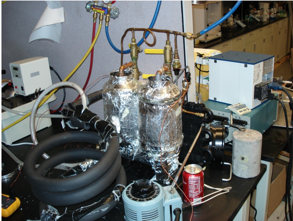
Figure 4.2. Adsorption system experimental set-up
