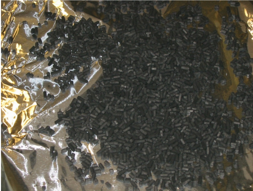
Figure 4.5. Activated carbon sample used as adsorbent in the adsorption system
