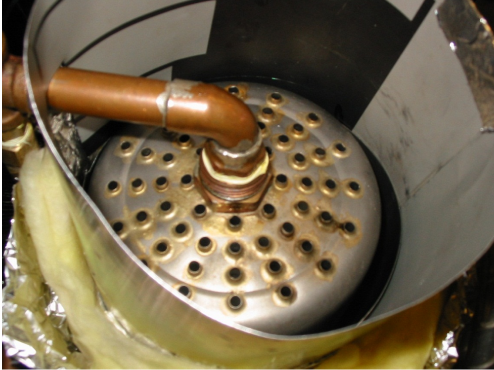
Figure 4.3. Top view of the adsorber vessel
