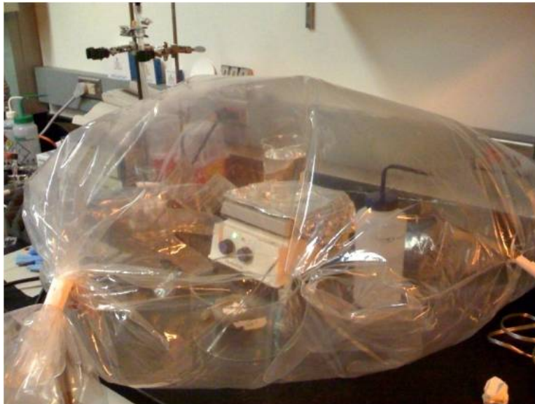
Figure 2.2. Glove bag set up used for incipient impregnation.
