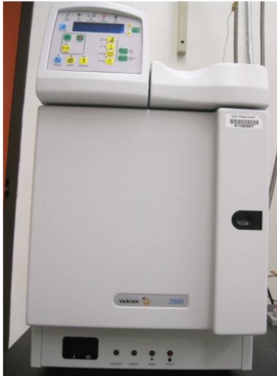
Figure 2.5. Varian 3900 Gas Chromatograph unit.
