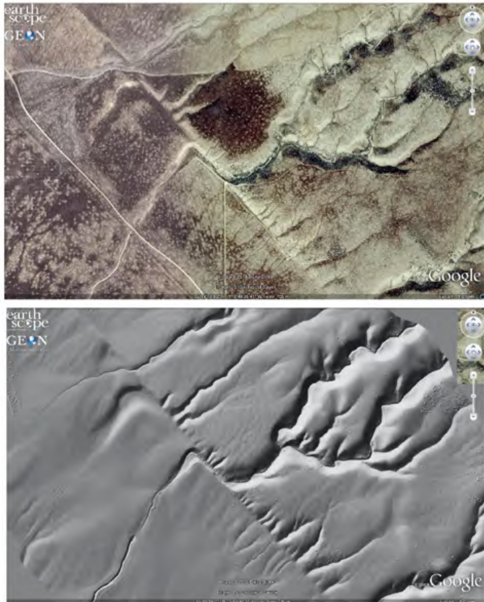
Figure 2. San Andreas Fault at Wallace Creek imagery. Google Earth aerial photography (top) and hillshaded LiDAR topography (bottom). For the distracter study, control students were given the aerial photography while experimental students were given the LiDAR topography in order to answer the same set of questions.
